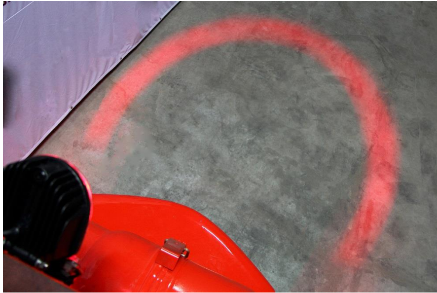
Overhead view of the Forklift Arch Light
